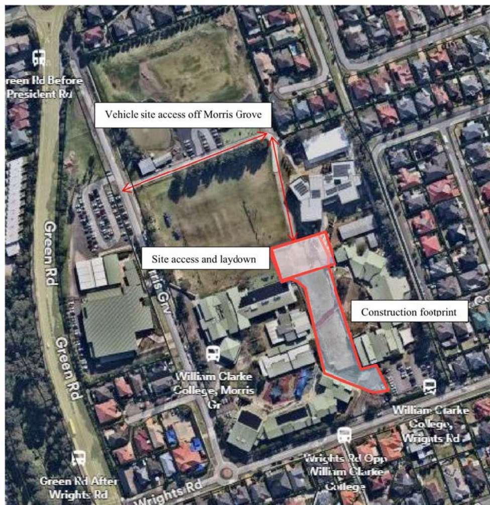
Figure 5-1 Site layout - Construction
